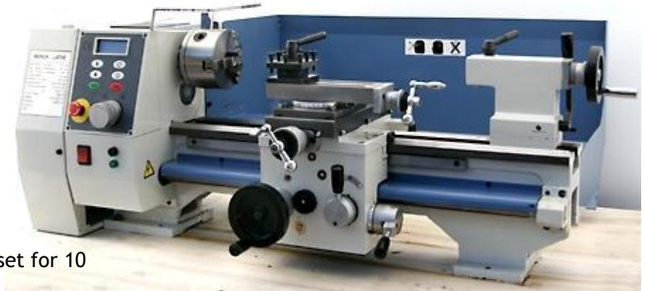
A reversible 2-mm pitch lead screw provides extended threading capability. You can create every American Standard Unified class 2A inch screw thread from 4 to 80 threads per inch, and you can create every American Standard Metric class 6h thread from 0.2 to 8 mm pitch with the change gears that are included.
